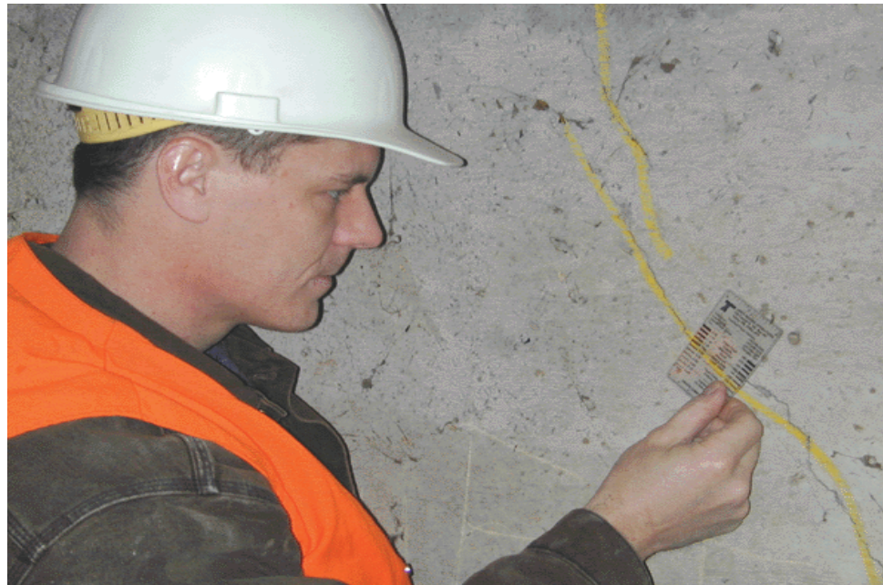
Figure 2.2.10 Crack Comparator Card
